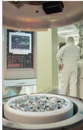
Quartz crucible filled with polycrystalline silicon
