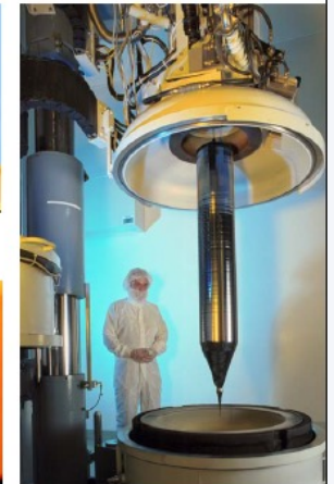
Single crystal silicon after CZ growth
